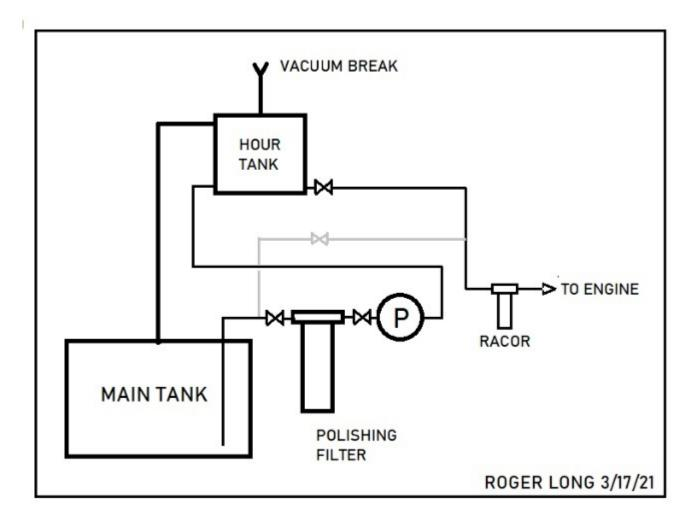
The Hour Tank is a steel or aluminum tank sized to approximately the engine's hourly consumption and located at or above the level of the mechanical pump on the engine. This will reduce the load on that component as the engine will be gravity fed. The return line at the top of this tank should be about twice the cross section area of the inlet piping from the pump and filter.
